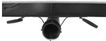
Black/Grey Tank Drain and Valves
