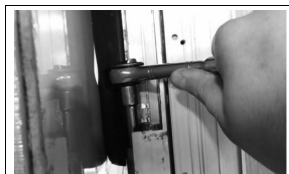
Figure 13 Ratchet inside motor access with socket on coupler
